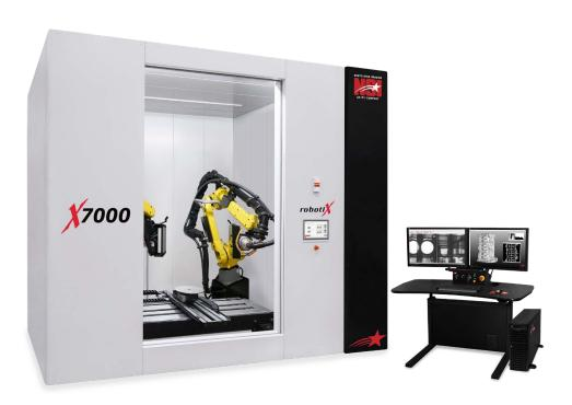
North Star Imaging's unique Dual RobotiX precision technology features two robot arms working in harmony of movement to scan large parts.
