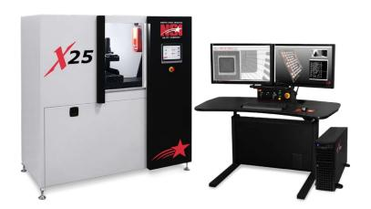
160 kV Maximum X-ray Energy 37 in [94 cm] Maximum Focal Distance
