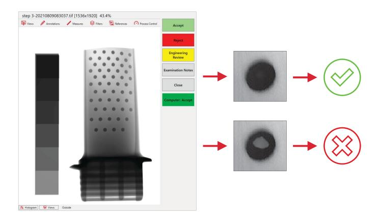
efX-ADR offers a simple and intuitive user interface that customers can easily set up and integrate into production workflows for automatic processing. Users can inspect high volumes of products and increase the reliability of interpretations. efX-ADR can help increase throughput, repeatability and can reduce costs. ADR provides a wide range of defect-detection mechanisms, and users can pick the ones that work best for their parts.
